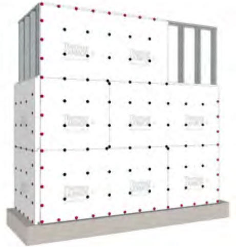
Figure 11: Fastening Pattern; Thermax™ Brand Exterior Insulation
